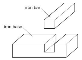
At room temperature, the bar is slightly too big to fit into the gap.
